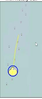
As noted, much of the received data is erroneous noise. LifeRing uses several processing algorithms that make automatic determinations that reject this noise data and only then applies an AGIS sensor algorithm to the remaining data to create track symbols which have speed and heading and, if available, altitude.
