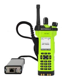
LifeRing provides an on-the-go, ad hoc network to be set up for all responders to join and immediately become part of a single responder group sharing and providing voice and data communications between them.
